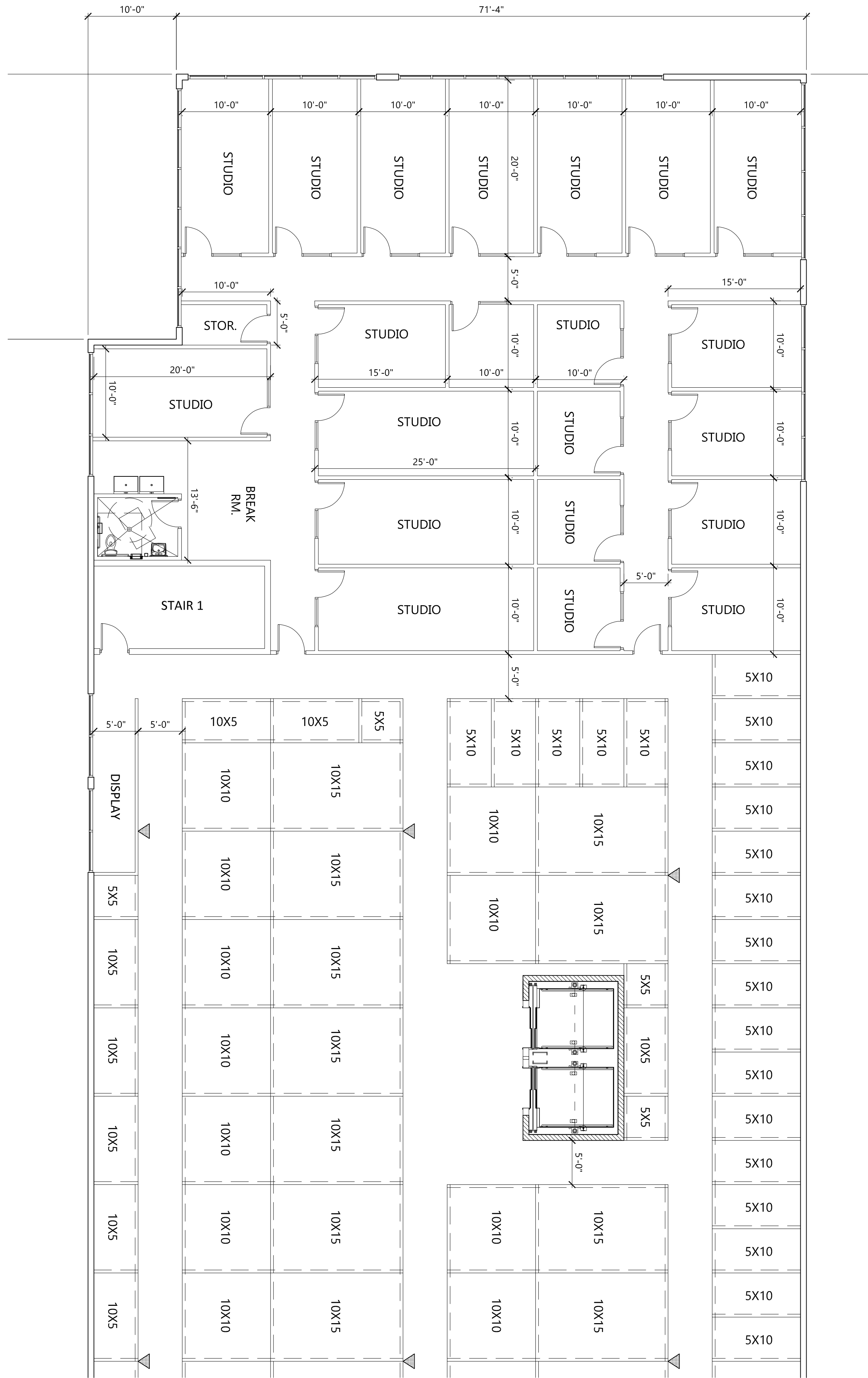
PARTIAL THIRD FLOOR PLAN SCALE: 1/8" = 1'-0"
